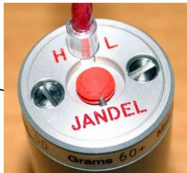
**Cylindrical Probe Tip Pressure** can be user adjusted within one of three ranges by turning the small knob on top of the probe towards either the "H" for higher or "L" for lower pressure.
