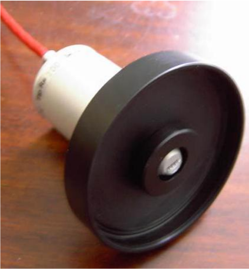
The Large Shroud installed on a Jandel Cylindrical Probe
