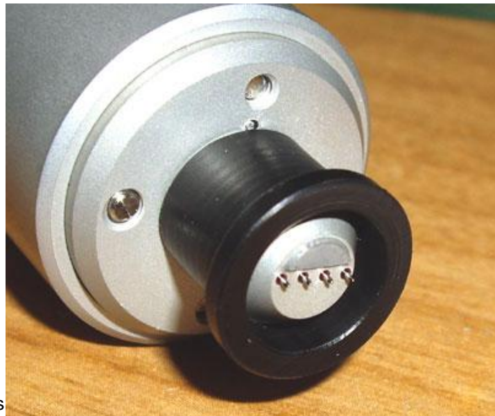
Small Shroud Mounted onto the Nosepiece of a Cylindrical Probe
